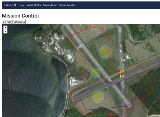
Figure 2: Early iteration of new custom GCS displaying the mission and current plane position.
